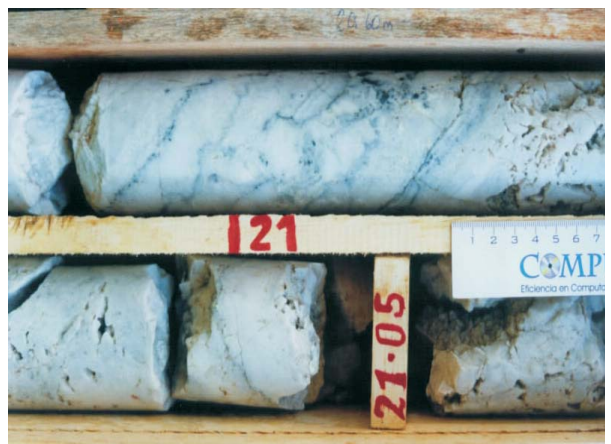
Banded quartz-sulfide veining in AngloGold drillhole DIVDDH-01 that graded 2 m @ 20.66 g/t Au and 69 g/t Ag from 20.26 m to 22.26 m
